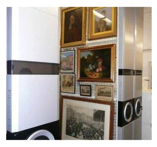
**Small Store -** This is adjacent to the Large Object Collection Store and houses the art and weaponry collection. Here there are 14 Manually operated mobile bases 3000mm long, each with an 'A' Frame 3300mm high, giving in total 277.20m2 of storage. The clever design of the 'A' Frame means that the paintings are 'canted' at an angle so that when the mobile units move none of the artwork 'flaps' against the mesh, something that is often associated with vertical mesh frame storage.
