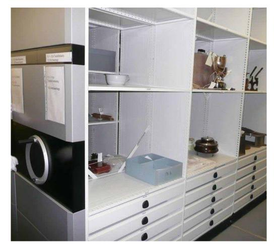
**Collections Access Area** - This is situated close by in an existing room, and is used to store Stockton Borough Council's archives and local history resources. The storage here consists of 5 Bruynzeel Manual mobile carriages 3.5m long x 3m high with shelves either 450mm or 500mm deep, one Gearwheel mobile with 'A' Frame for artwork storage and one single sided Gearwheel mobile with a decorative back and Floor-lock for security purposes.
